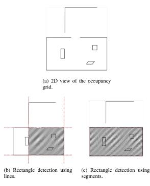
Fig. 2. Rectangle detection using the variation of the Hough transform based on lines (b) and the proposed one based on segments (c).
