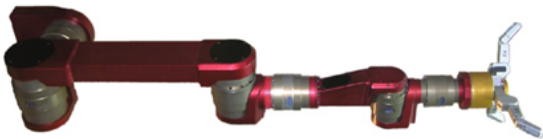
Fig. 13: Loki's initial arm with a Barret hand
