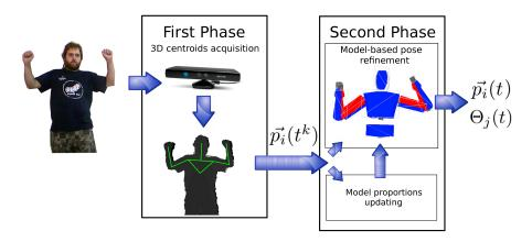
Our HMC system has been quantitatively evaluated through two sets of experiments. Experiments in the first set measure limb lengths and instant position errors for different arm gestures, using a commercial, multi-view marker-based system as the ground-truth. The second set of experiments evaluate the percentage of correctly estimated joint positions in a set of labeled motion sequences. The results obtained are deeply discussed in the following sections.
