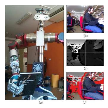
Fig. 3. a) PrimeSense sensor (kinect style) mounted on the Muecas robot head; b) RGB image acquired by the RGB-D sensor; c) depth information associated to the RGB image shown in b); and d) RGB image after callibrating.
