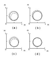
Fig. 2. (a)–(d) Fits to a set of range readings (grey points). Encoding is Zhang *et al.*'s approach [3]: dotted and Bailey's approach [7]: dashed; Proposed method: solid.
