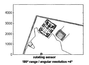
Fig.12 Ultrasonic perceptual environment
