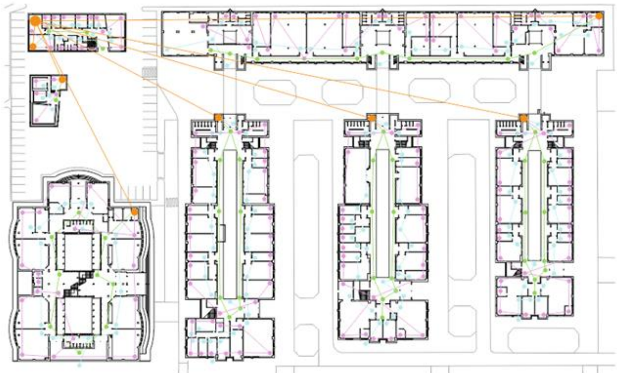
Fig. 2: Proposal of sensorization provision for the Smartpolitech project
