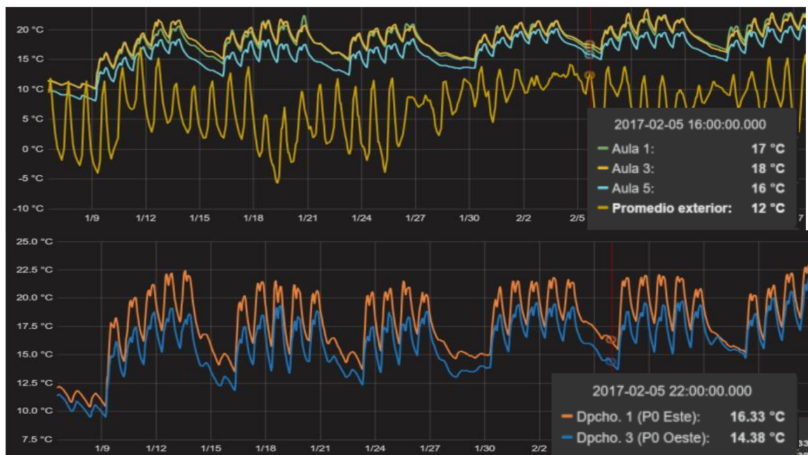
Fig. 4: Graphs of the thermal behaviour in different floors in School of Technology
