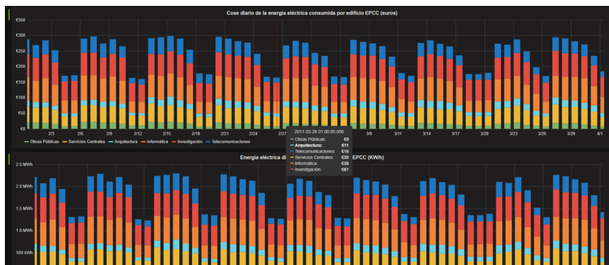
Fig. 8: Graphs of the economic cost of the electric consumption in different buildings in School of Technology
