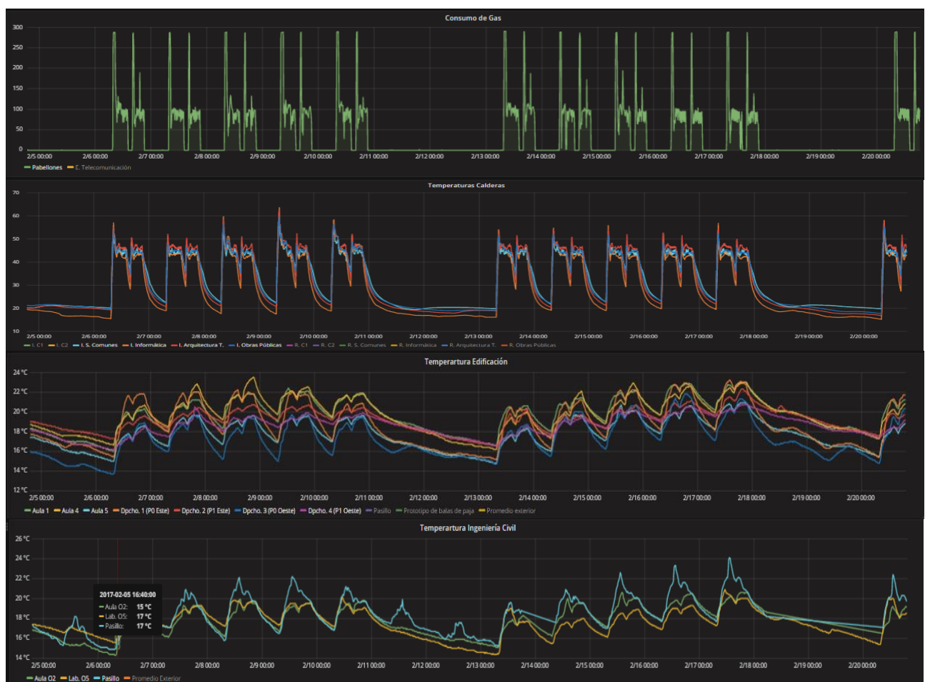
Fig. 5: Graph of gas consumption in heating system; and graphs of boiler temperatures, and indoor temperatures in different buildings in School of Technology.
