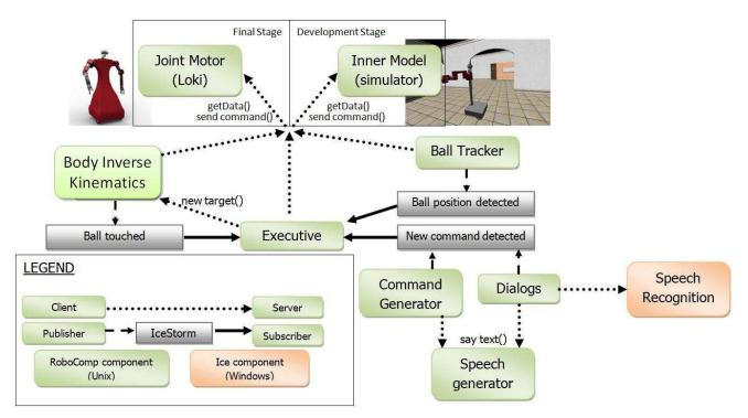
Fig. 4: Global system architecture. The drawing shows the main components of the architecture and the type of communications that occur among them.
