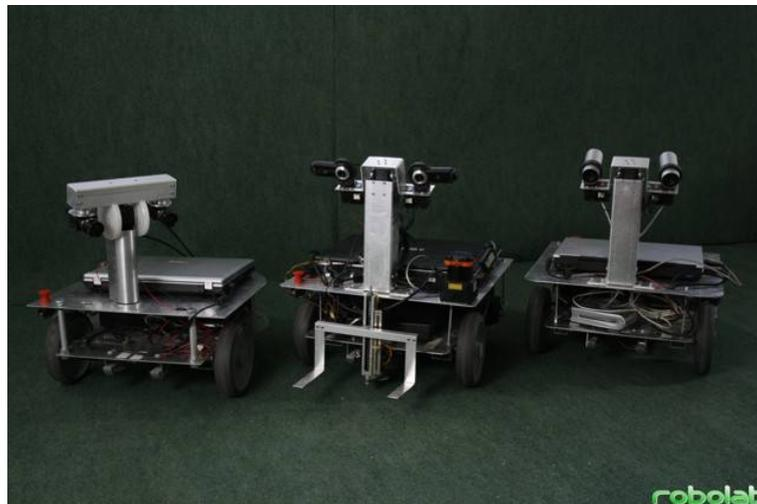
**Figure 1.3:** The three Robolabs robots using the RoboEx platform. The central robot, in addition to the rest of devices, has mounted a forklift
