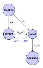
Fig. 2. Unified representation as a multi-labeled directed graph. Edges labeled as is\_with and is\_not denote logic predicates between nodes and they belong to  $\Gamma_s$ . Edges starting at **room** and ending at **person** and **robot** are geometric and they encodes a rigid transformation (RT' and RT respectively) between them. Geometric transformations can be chained or inverted to compute changes in coordinate systems.
