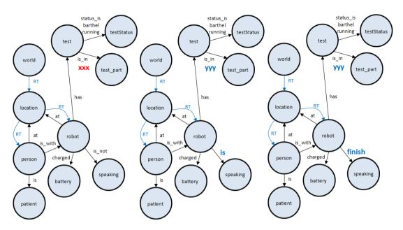
Fig. 3. (Left) The state of the DSR before PELEA states that the robot should say a sentence **yyy**; (center) PELEA changes the text to speech (from **xxx** to **yyy**) and then, when the Speech agent reads the DSR, the robot starts to speech (**robot** is **speaking**); and (right) the sentence has been said and the Speech agent informs to the rest of the agents through the DSR (**robot** finish **speaking**).
