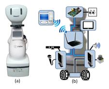
Fig. 4. (a) Gualzru, the robotic salesman; and (b) Hardware structure
