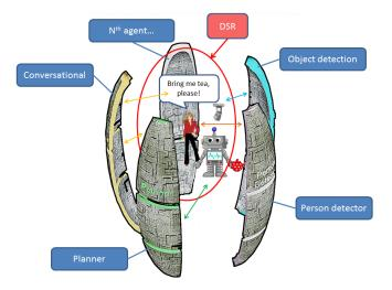
Fig. 2. Overview of the CORTEX architecture depicted as quasi-cylindrical shape sliced in agents with the shared representation occupying the central volume.
