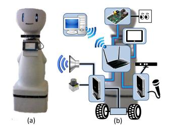
Fig. 2. (a) Gualzru, the robotic salesman; and (b) Hardware structure
