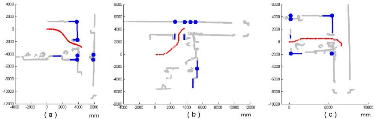
Fig. 5. Several tests in the same environment following different trajectories. The spectral clustering algorithm generates the same submaps in each experiment. When the robot leaves the room and enter in the corridor the thresholds values for  $N_{cut}$  and the second eigenvalue are satisfied.
