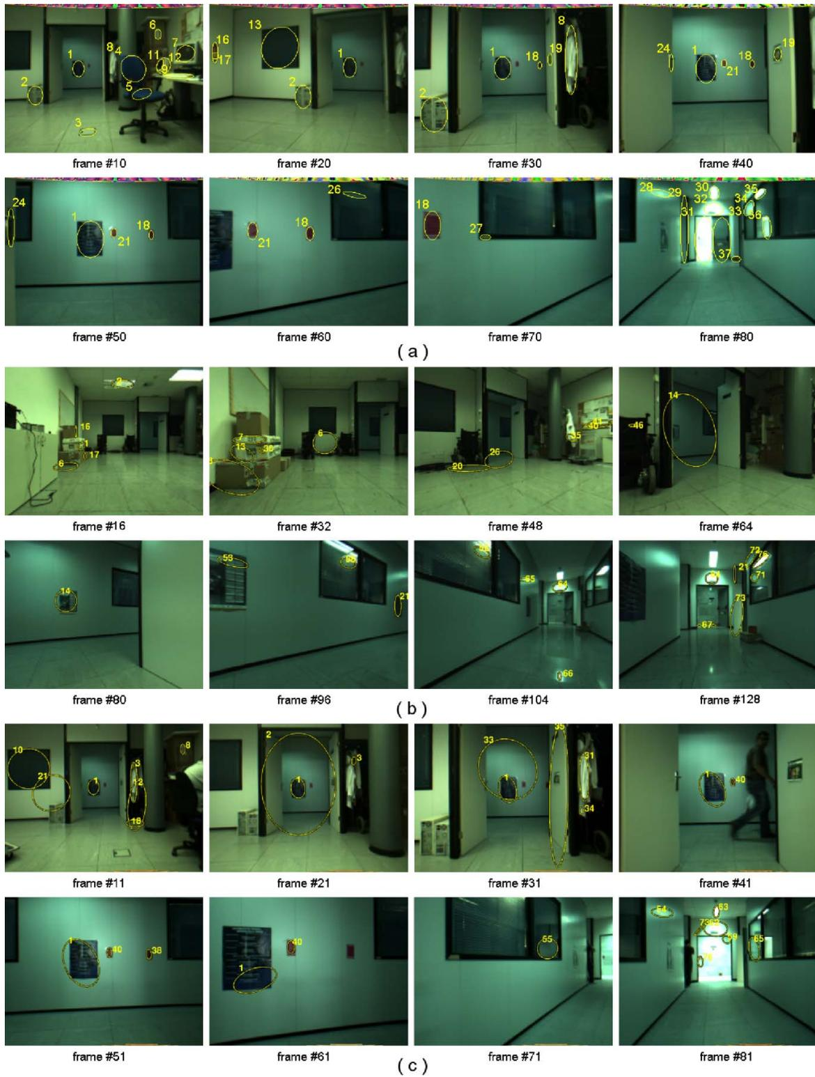
Fig. 7. Some experiments using vision. Three experiments in the same scenario in different viewing conditions. Visual landmarks detected are represented as ellipses, and the correspondence between landmarks in different frames with the corresponding index. A new area is detected at the same location as for the laser experiment. a) new area detected in frame #70, b) in frame #104 and c) in frame #71.
