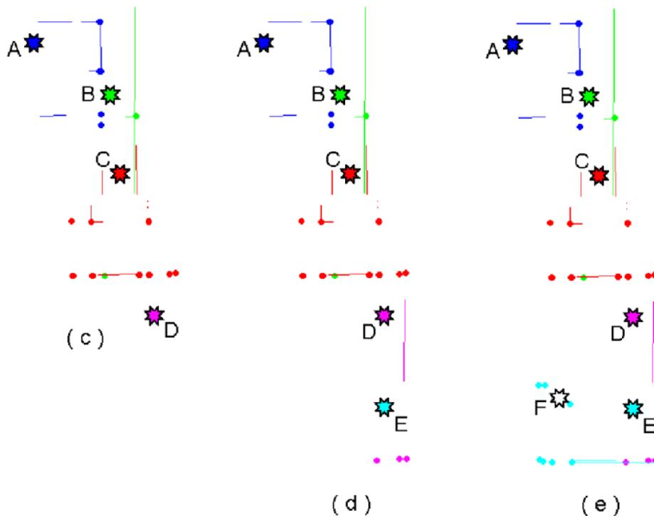
Fig. 6. Experiment in a real indoor environment with a laser range finder. a) Environment layout; b) detected submaps; c) submaps generated during the trajectory up to the third cut, d) and e) following partitions in the trajectory. Features have been obtained using a curvature-based laser scan data segmentation algorithm [17].
