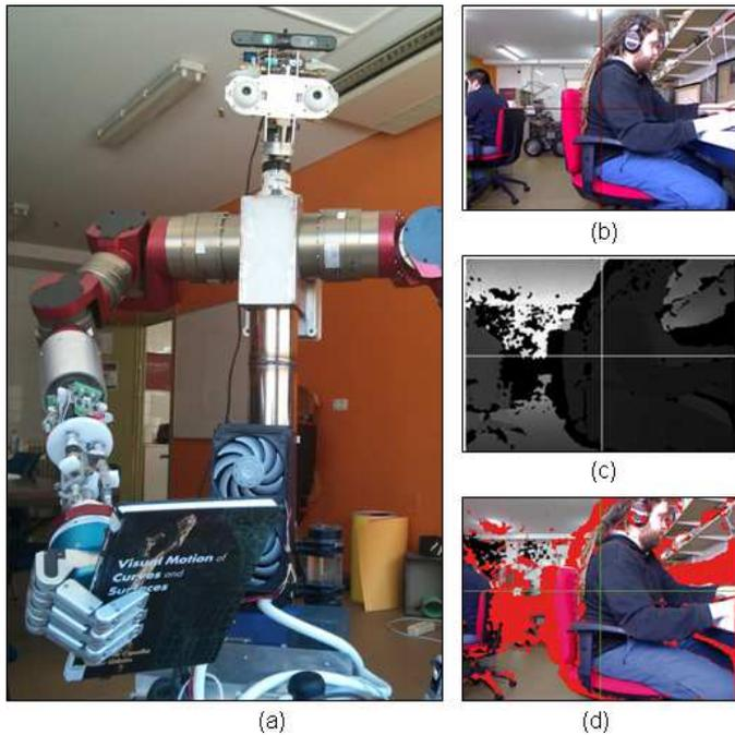
Fig. 3. a) PrimeSense sensor (kinect style) mounted on the Muecas robot head; b) RGB image acquired by the RGB-D sensor; c) depth information associated to the RGB image shown in b); and d) RGB image after calibrating.
