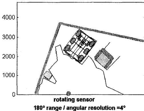
Fig. 12 Ultrasonic perceptual environment
