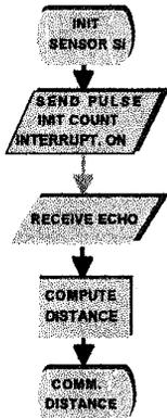
Fig 8 Single event processing flow
