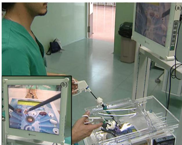
**Fig. 6** This photograph shows the testing conditions of the experiment: **a** Surgeon performs a training task with the EDEST device and **b** Screen shot of the monitor view
