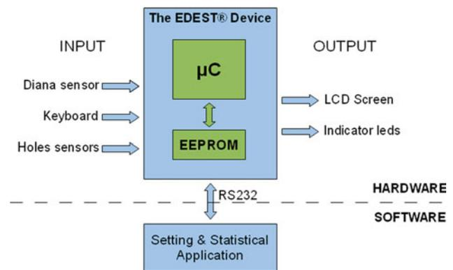
**Fig. 2** General view of the EDEST® device: main components, I/O system and communication port
