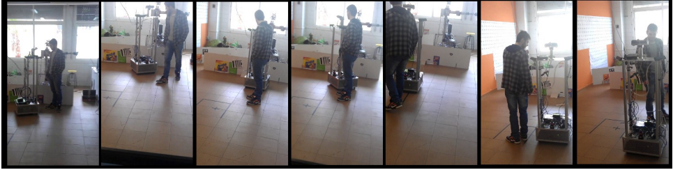
Fig. 9. The robot moves towards its goal while avoiding a moving person.
