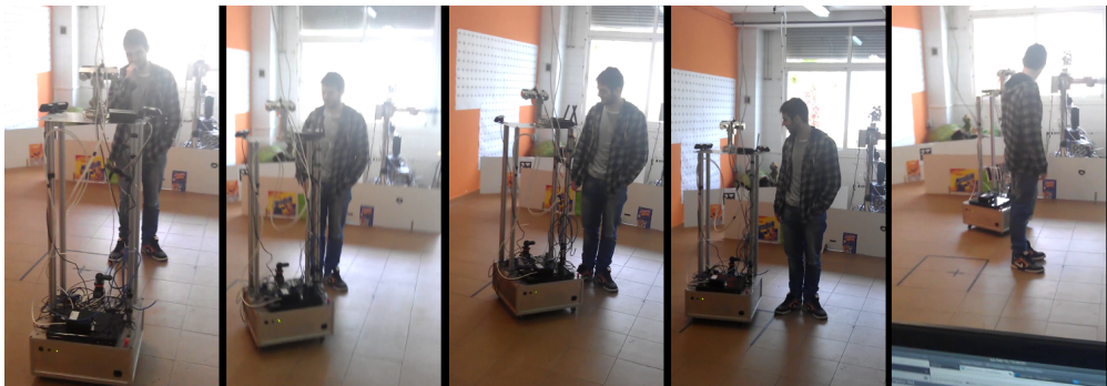
Fig. 8. The robot moves towards its goal while avoiding a standing person.
