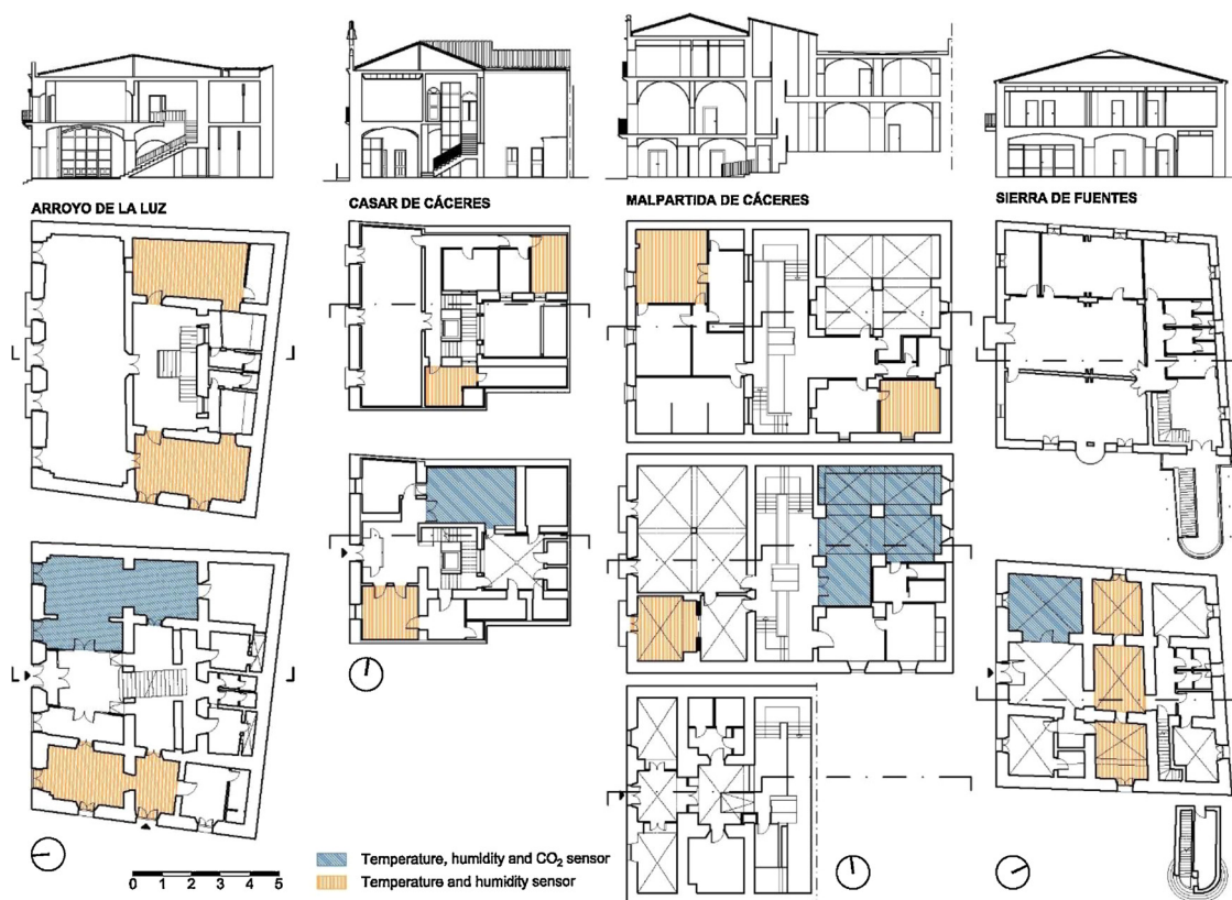
Fig. 3. Town Halls interior design and location of the sensors.
